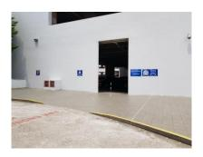
A kerb will be built at the entrance to reduce rain water flowing into Plaza driveway.
